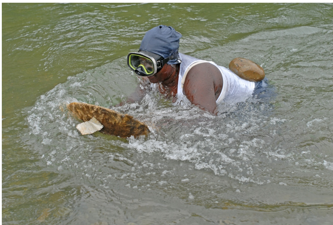
Figure 2. Zambuyidero or diving technique. Artisanal method used in prolonged summer periods, when river levels drop. The gold is located at the bottom of the river and the miner makes successive dives to take out the gold and platinum containing material which is washed using a pan. Photograph by Kike Arnal.
