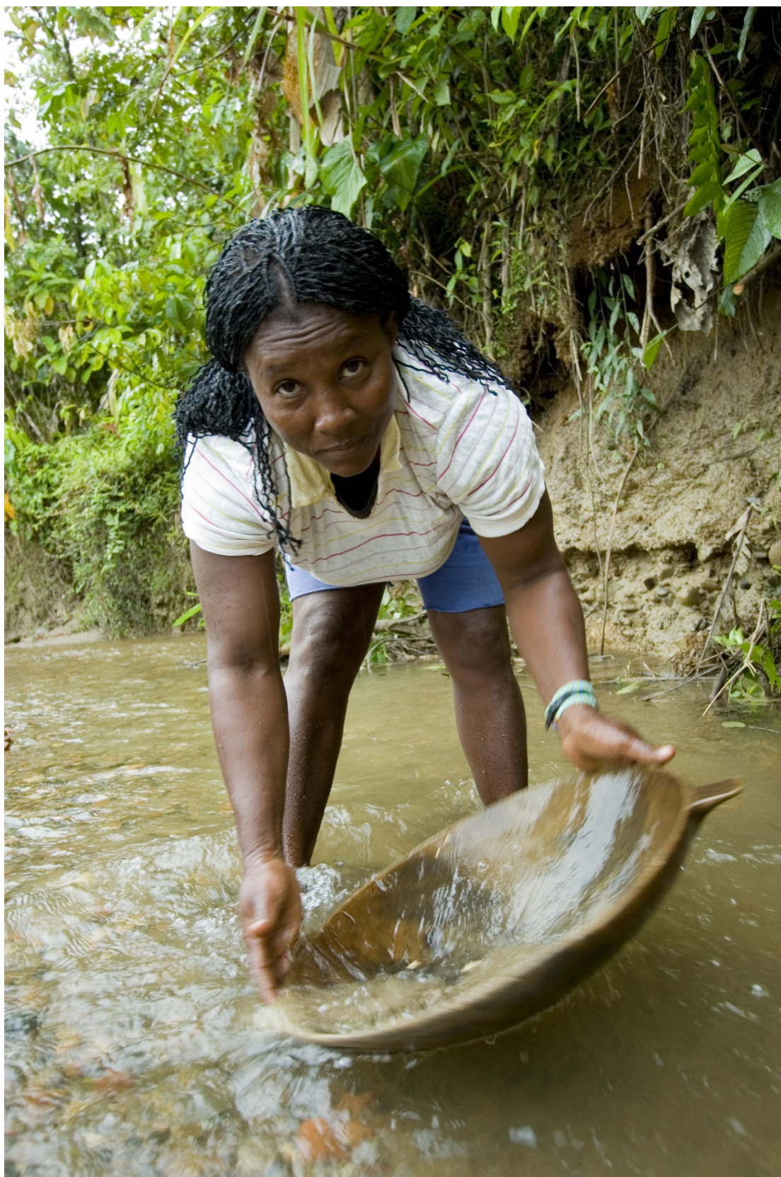
Figure 1. Mazamorreo or panning technique. Artisanal method that involves getting the gravel from the riverbeds and the gravel banks of the rivers, which is washed in the pan until the gold and the platinum appear. Photograph by Alejandro Cock.
