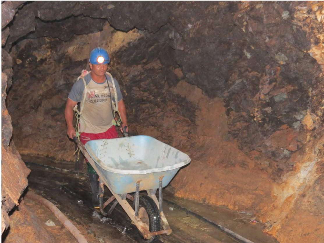
Figure 4. Los guaches, hoyadero , or underground mining, one of the most common techniques in the Chocó area. It is an excavated pit, with walls held by wooden poles. The depth of the holes depends on the distance of the place where the gold and the platinum are located, but can be up to 15 meters deep. Photograph by Oro Verde.
