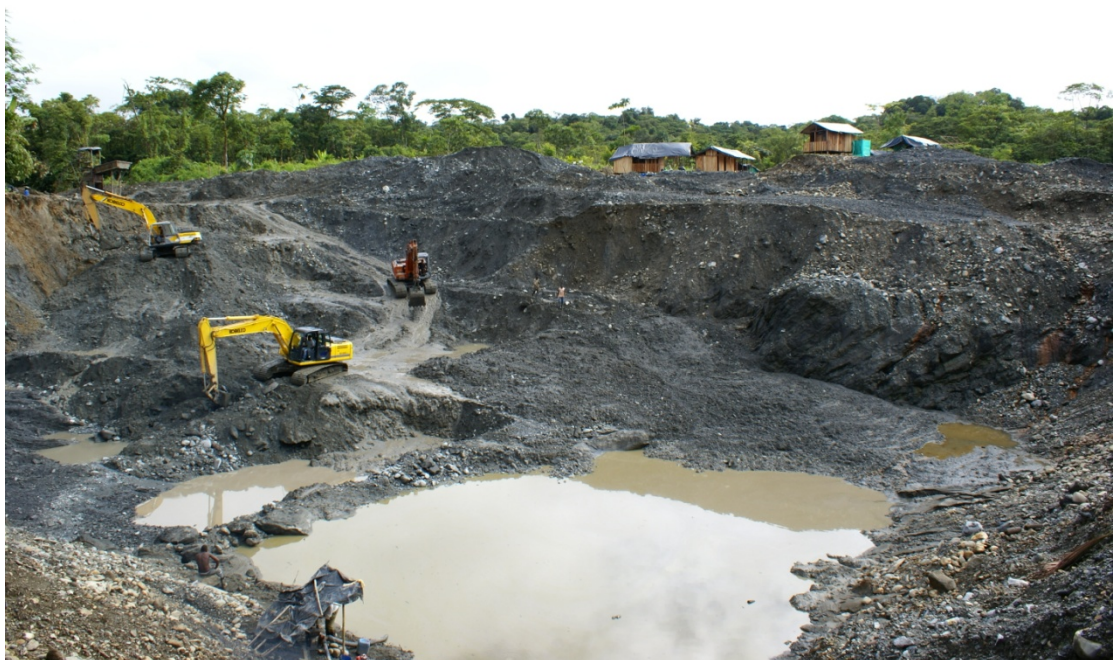
Figure 5. Small-scale mechanized mining. This is mining that uses mechanized equipment, such as small suction dredges, water pumps, sluice boxes, hydraulic excavators, and suction and spoon dredges. Photograph by Oro Verde.
