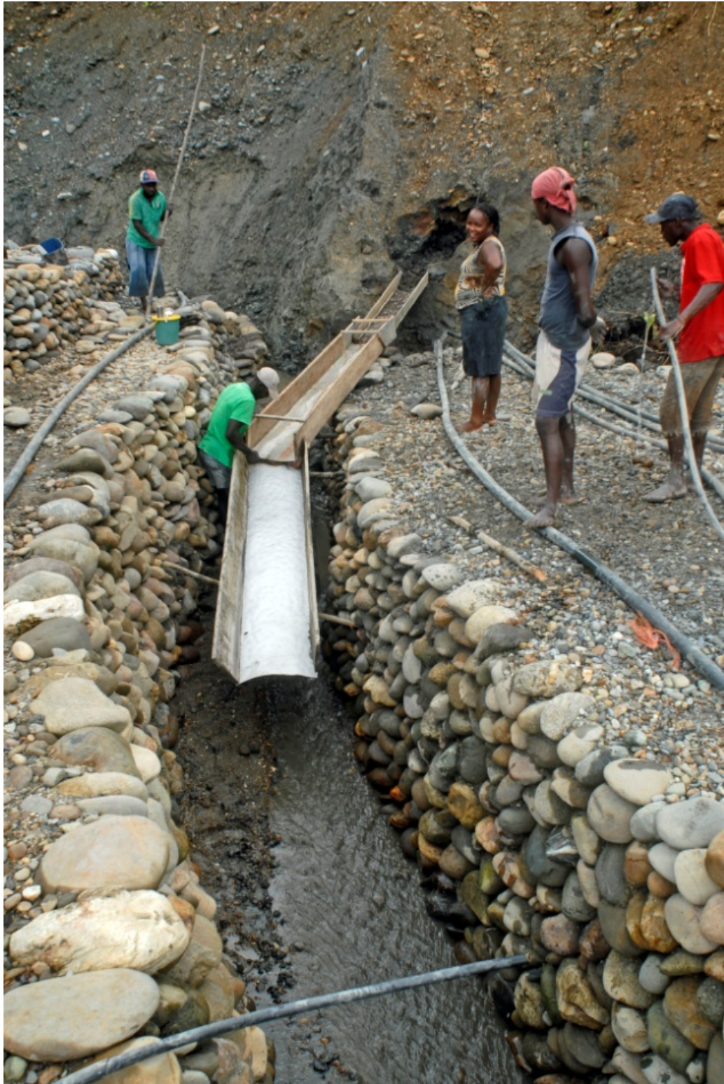
Figure 7. Agua Corrida . Artisanal mining method performed by Afro-Colombian communities where sands are washed utilizing water pressure. Ponds, gravity and occasionally small water pumps are utilized for creating pressure. Photograph by Oro Verde.
