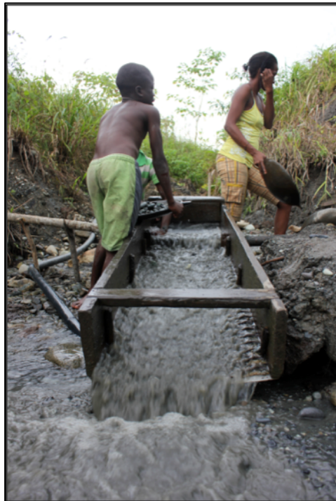
Picture 8 and 9. Separating gravel from gold through the canalón
