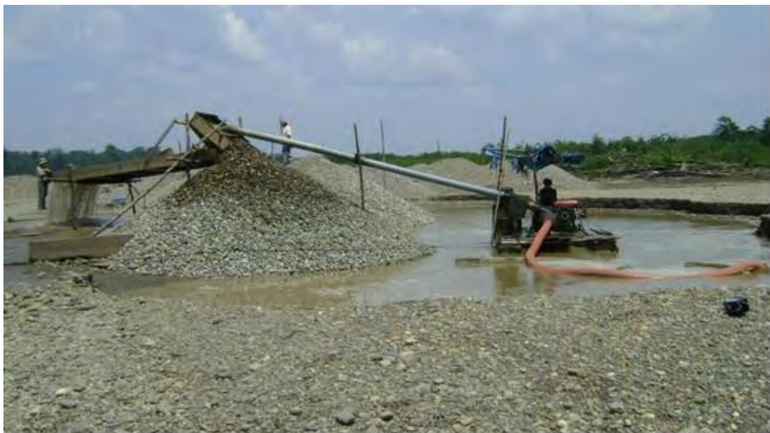
Picture 4.1. Miners using the “ caranchera ” (suction pump) to extract gold from the riverbed. (Source: Mosquera et al. 2009)
