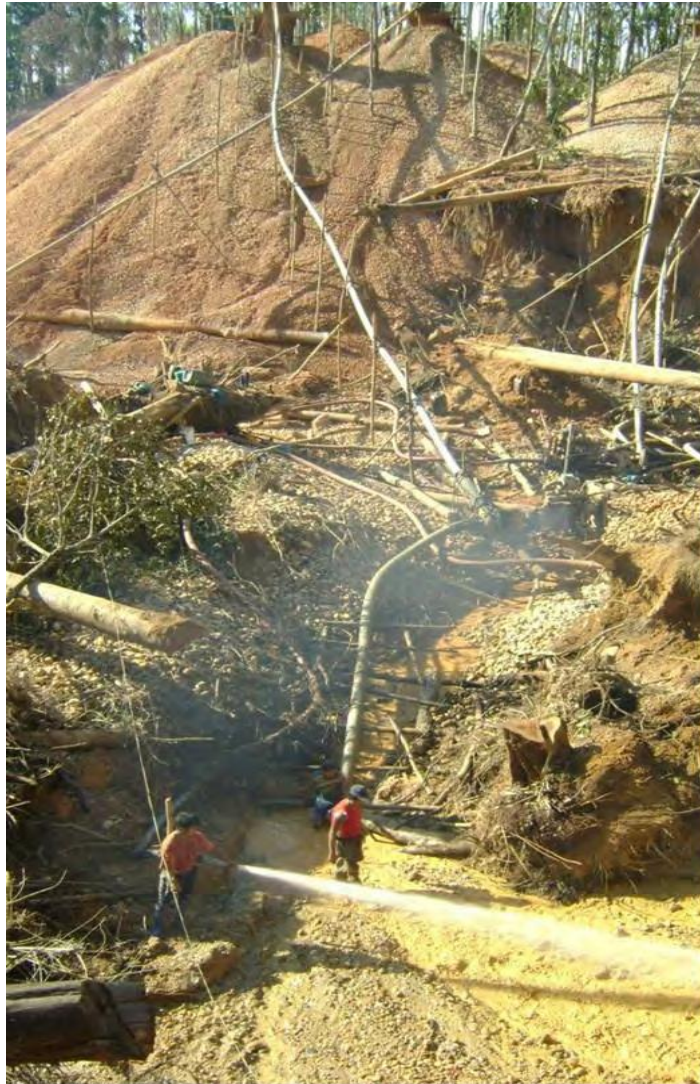
Picture 4.2. Miners using the “chupadera”(vacuum pump) for exploiting gold deposits in the forest. (Source: Mosquera et al. 2009)
